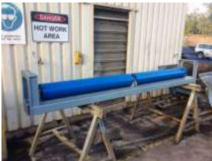
Image 4: Two piece roller to reduce weight and make the rollers easier to handle
