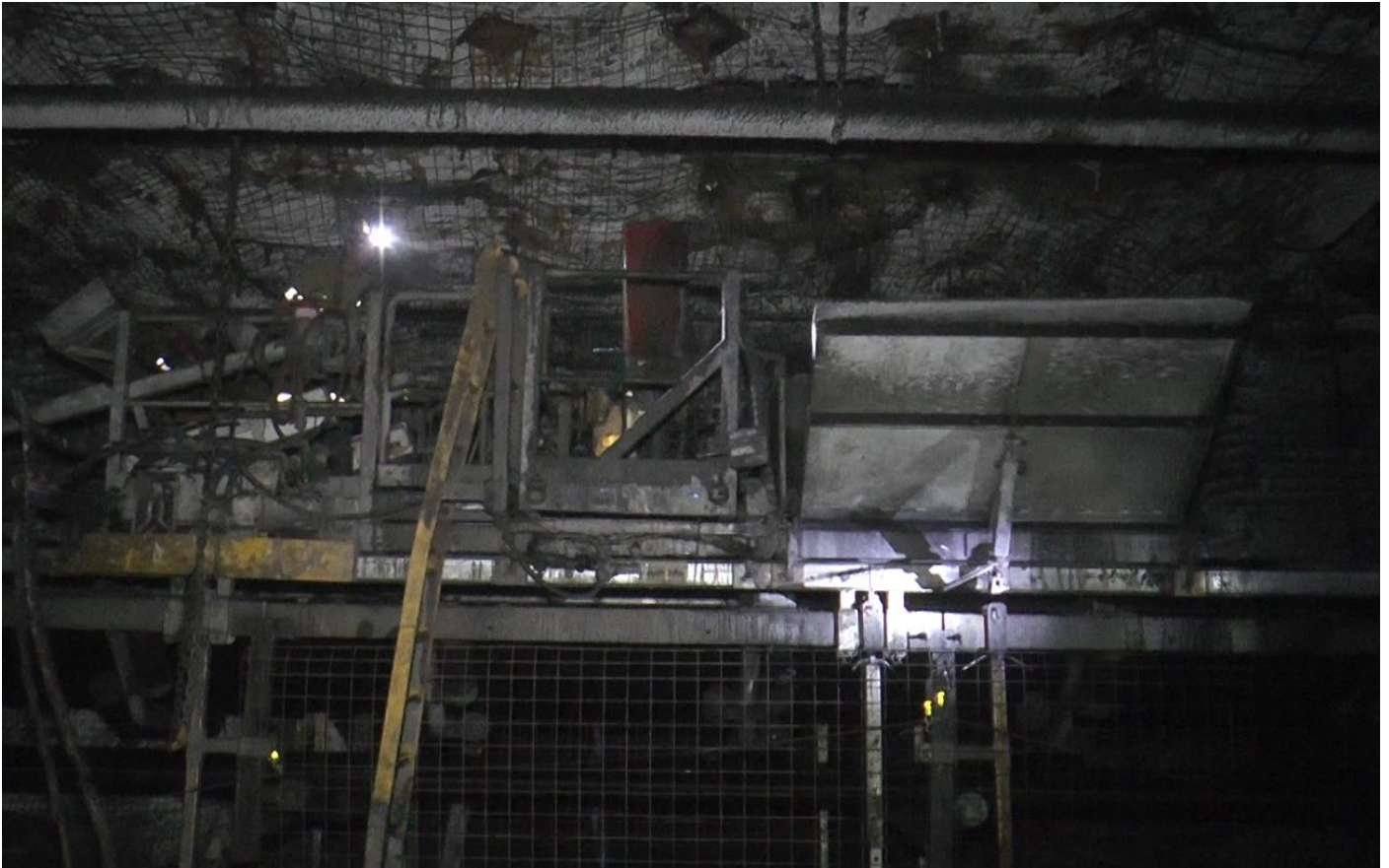
Bolter positioned and operational over TC01 main trunk conveyor.
