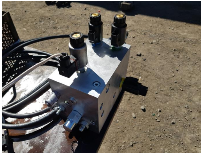
Picture 2: External Pump Control
