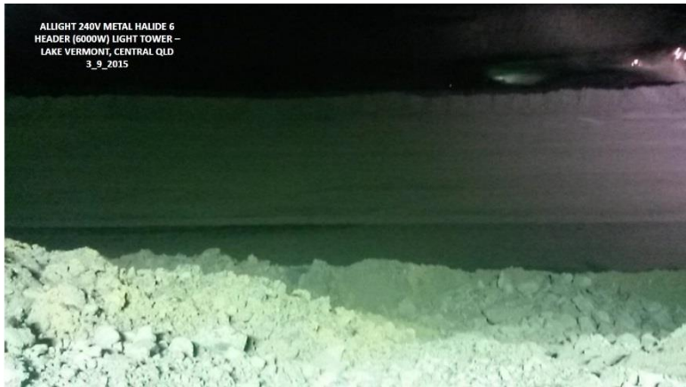
Figure 2 240V Lighting Output
