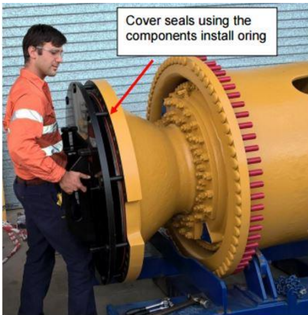
Figure 2: Version 2 - HDPE Final Drive Cover with fold-away handles
