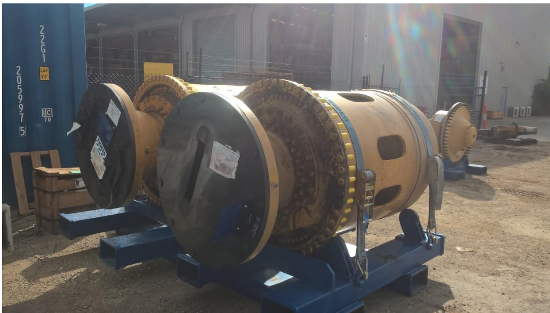
Figure 3: Version 3 - HDPE Final Drive Cover with in-built box
