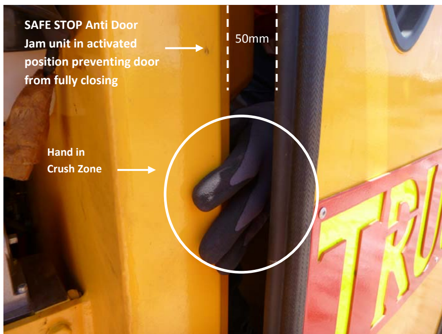
Picture 5: Operators have a tendency to position hand on cabin pillar when exiting cabin, this creates a crush hazard when door self closes due to machine being positioned on an angle or gradient in underground Environment.
