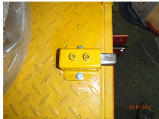
Picture 5: Operators have a tendency to position hand on cabin pillar when exiting cabin, this creates a crush hazard when door self closes due to machine being positioned on an angle or gradient in underground Environment.
