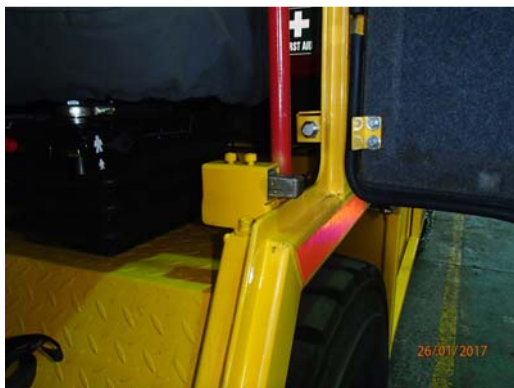
Picture 5: Operators have a tendency to position hand on cabin pillar when exiting cabin, this creates a crush hazard when door self closes due to machine being positioned on an angle or gradient in underground Environment.
