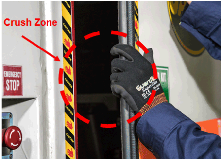
Picture 1. Potential Crush Zone in cabin door jam area when operator closing door from outside of cab
