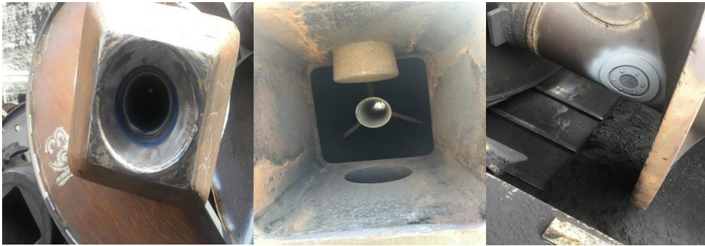
Picture 4 - Gas tube shank, socket and delivery port
