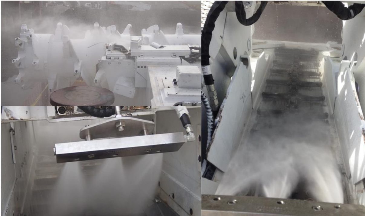
Figure 2 – Enviromist 100 Bar spray Circuit
