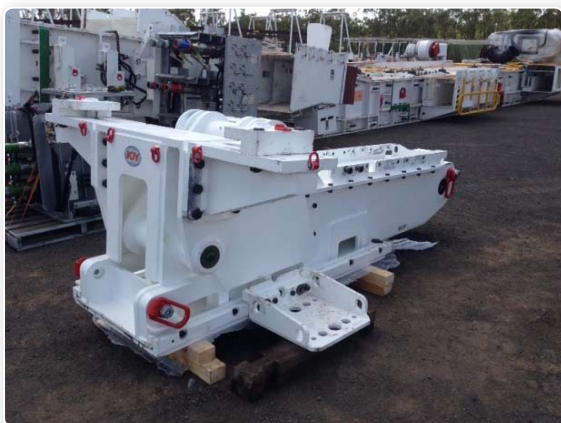
Figure 3 - Assembled Lifting Aid ready to be placed under BSL section
