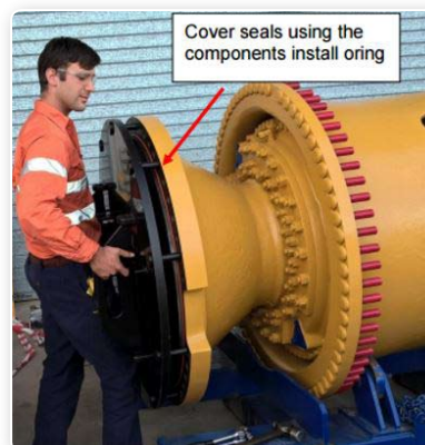
Figure 2: HDPE Final Drive Cover - Prototype two featuring fold-away handles
