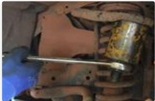
Figure 3: Ball Joint Installation Puller
