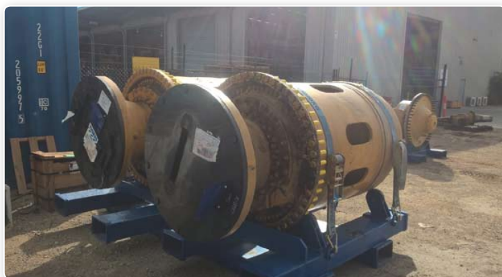
Figure 1: HDPE Final Drive Cover - Final Prototype with in-built box
