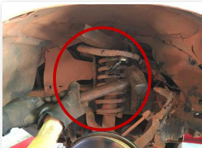
Figure 1: Tradesperson using a heavy hammer to strike to force the ball joint out
