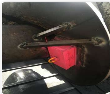
Picture 1 - Gas monitor mounted on auger cutter head
