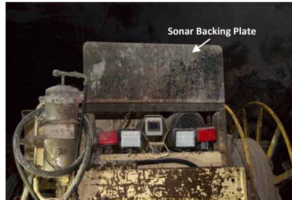
Picture 6 - Sonar backing plate fixed to spray rig.
