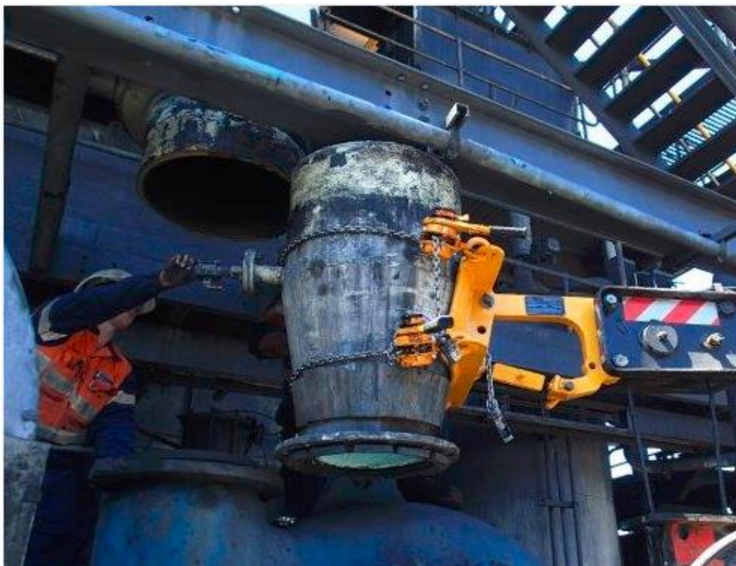
Fig.5 New Acland Coal's Multi-Fit Pipe Lifting Attachment shown in the process of removing a discharge spool from a XG-350 Metso Pump.
