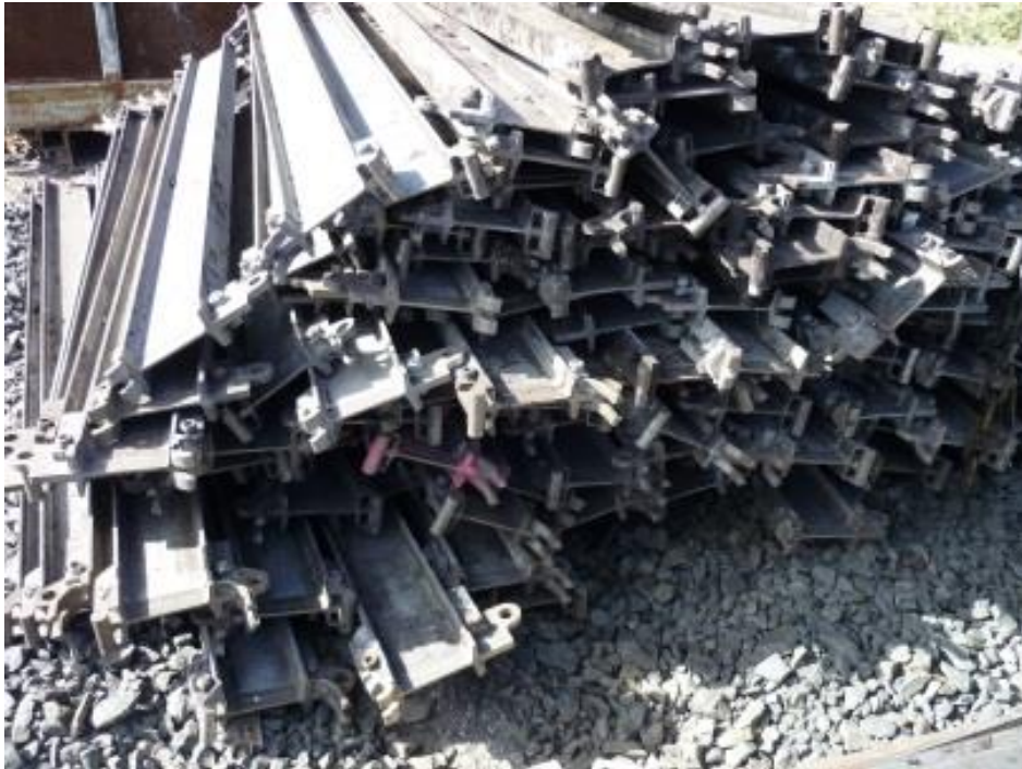
Example of how beams were previously stored, with obvious potential for damage to ends.
