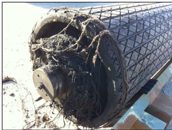
FIGURE 1: Buildup of string on pulley
