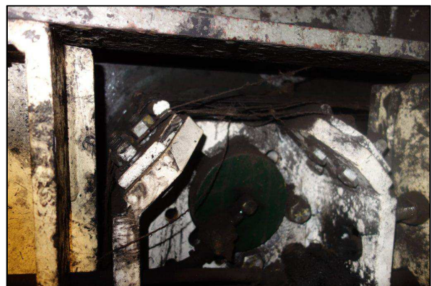
FIGURE 3: String gathering on 'pulley string catcher'
