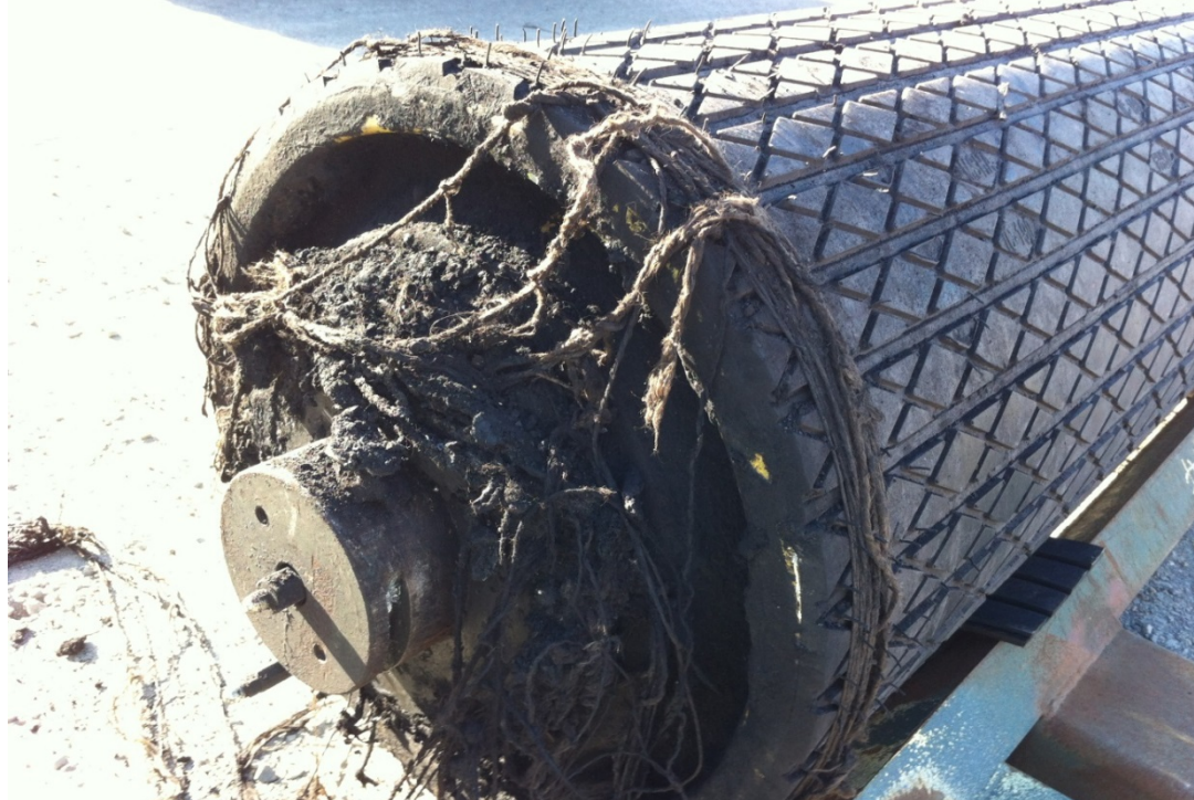
Failed Moranbah North Pulley due to string ingress
