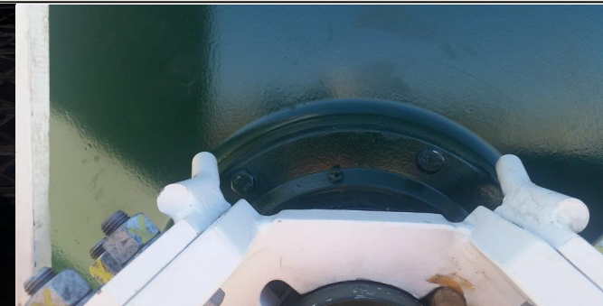
Pulley String Catcher installed on the loop take up pulleys before installation underground
