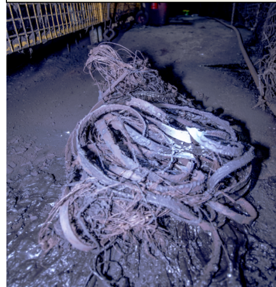
String and rubber removed from pulley seals underground
