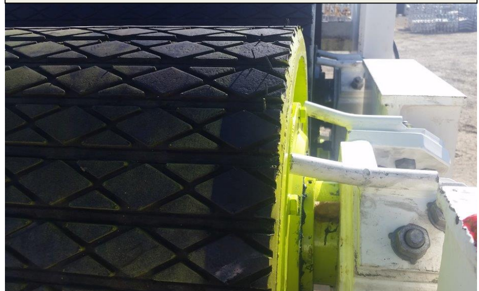
Pulley String Catcher installed on loop take up pulley before installation
