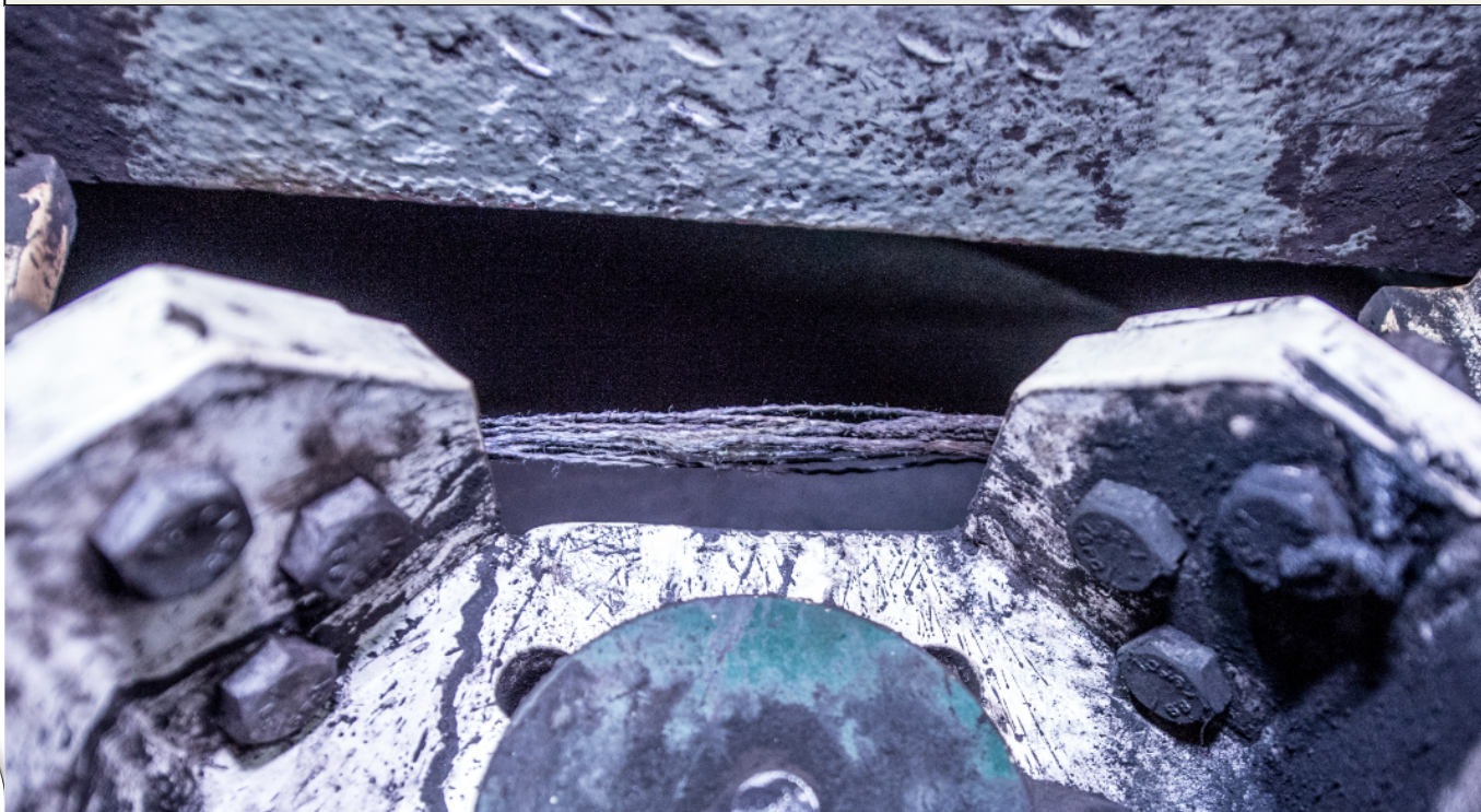
Pulley string catcher installed underground removing string from the belt
