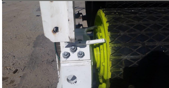
Pulley String Catcher installed on the loop take up pulleys before installation underground
