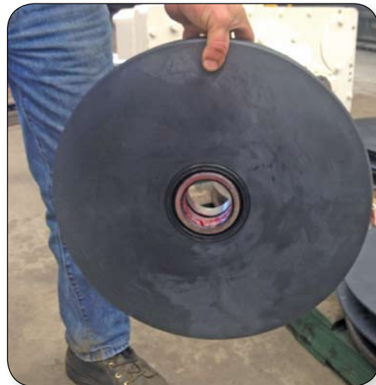
Figure 2. Maintainer holding the 10kg Nylatron sheave
