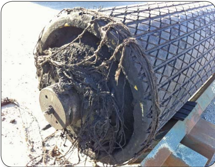
FIGURE 1: Buildup of string on pulley shaft
