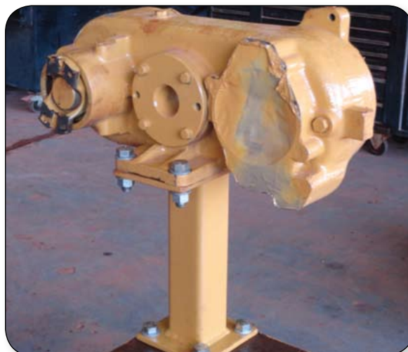
Figure 2: Pump drive box assembly on support stand.
