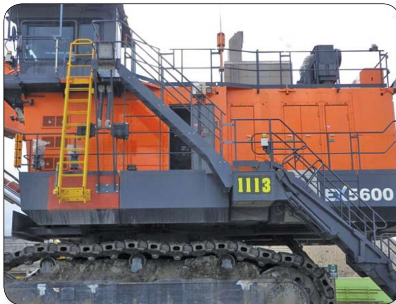
Photo 2 – New Access System Installed
