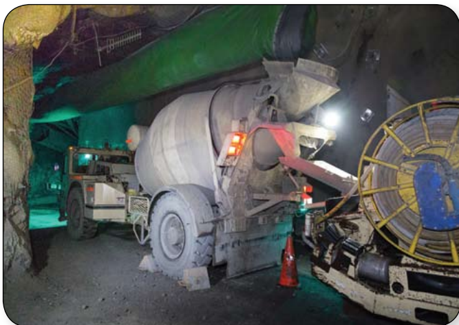
Picture 1 - Agitator discharging load using sonar discharging system.
