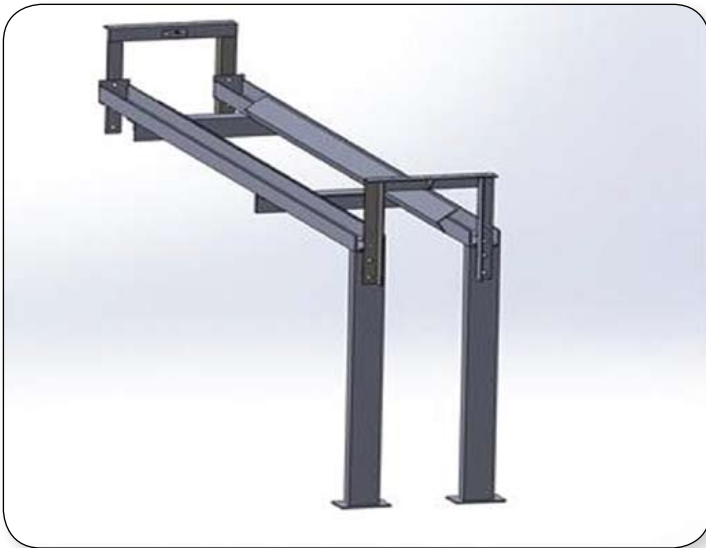
Figure 1: Pulley removal frame drawing.
