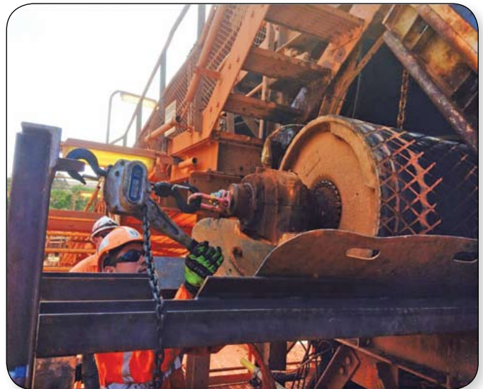
Figure 2: Pulley removal frame in use.
