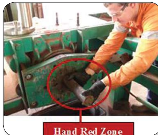
Figure 1: Main workshop personnel demonstrating how the extension pieces were held in place by hand and leaning over press.
