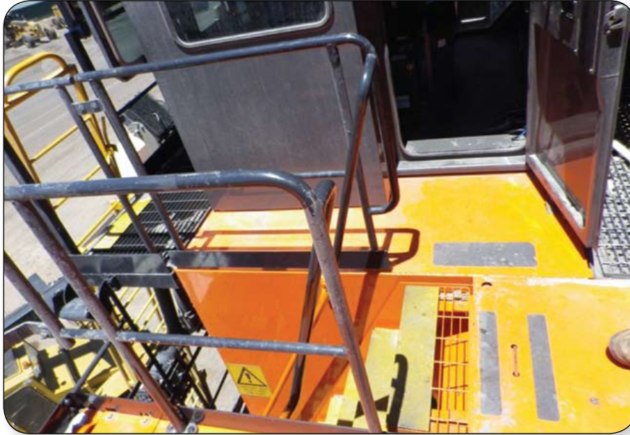
Photo 1 – Original Hitachi EX5600 Excavator Access System
