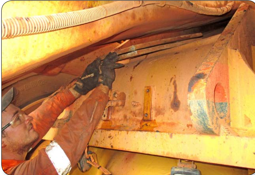
Figure 1: Fitter placing the plates between the loader and the boom
