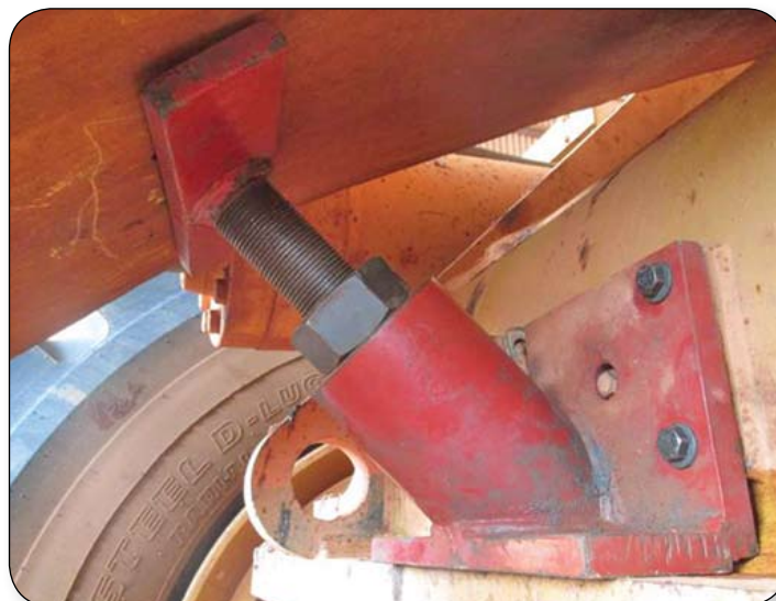
Figure 2: Loader boom adjustable support tool innovation
