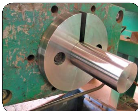
Figure 2: Self-supported press plate and extension piece.
