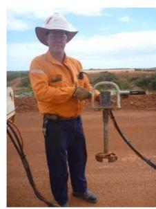
Figure 2 Hydraulic valve opener tool
