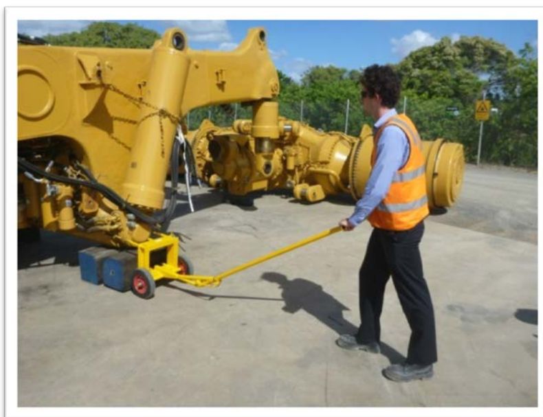
Figure 1 – A risk assessment found back injuries were a high probability when manually handling 50 kilogram-plus timber blocks.
