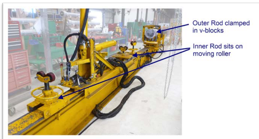
Figure 1 — Cylinder assembly bench general layout: original roller assemblies shown.
