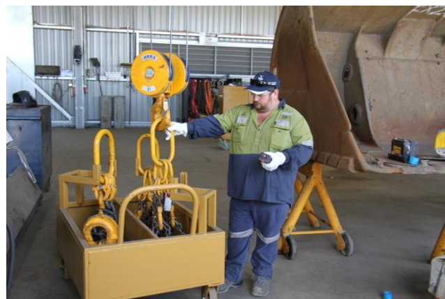
2. The chain can then be hoisted directly off the trolley, with no manual handling required.
