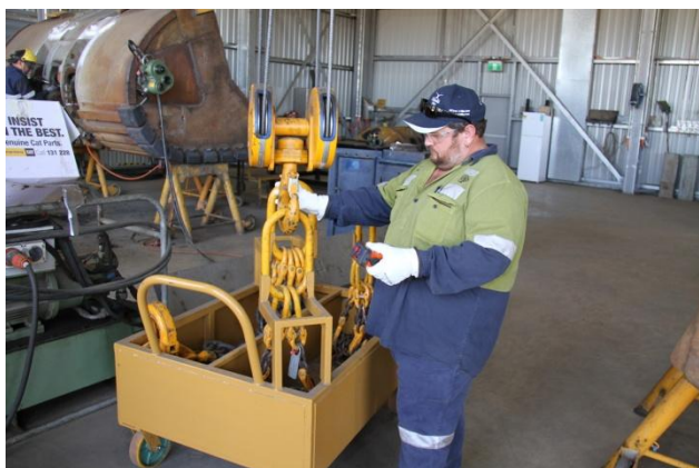
1. The trolley allows the crane hook to be lowered and clipped directly onto the chain's bull ring, requiring <math><2\text{kg}</math> force.
