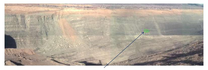
Radar file from May 2013 showing two pixels that had been activated by Minor Fall of Ground – in this case, an alarm was not required due to the ability of the physical controls to contain all of the material
