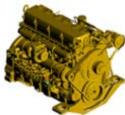
Existing underground loader engine
