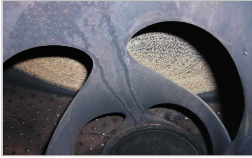
Figure 1. Intake of the diesel particulate flow through filter developed for the R1700G and R2900G engines.
