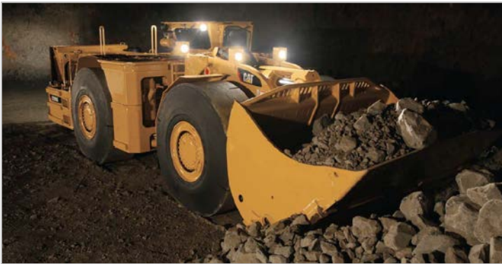
Figure 4. Test machine R2900G loader at Cannington.
