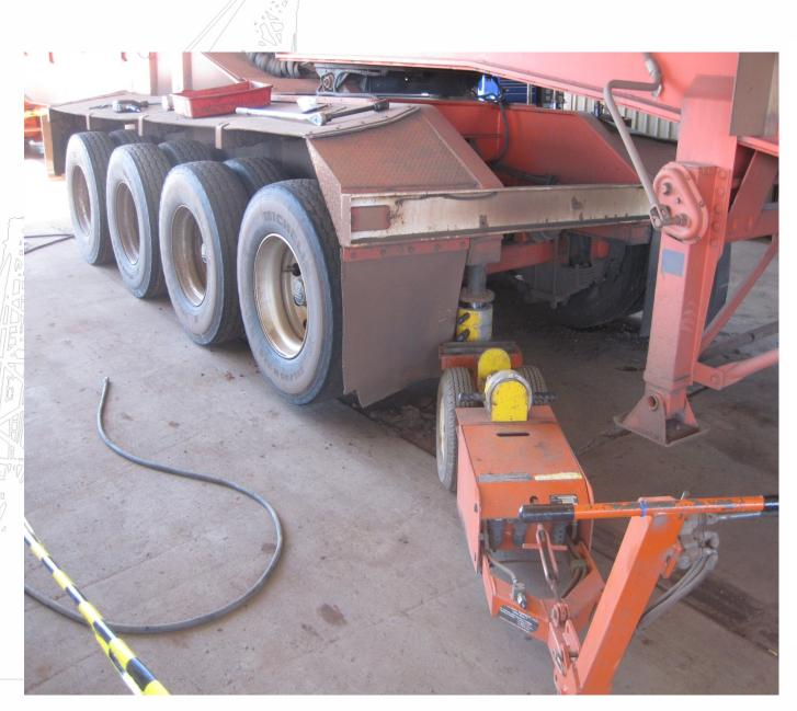
The axle is raised off the ground by supporting the bogey chassis.
