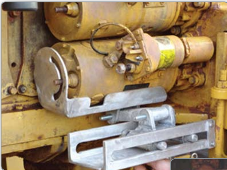
Figure 1: Starter motor jig being bolted into place
