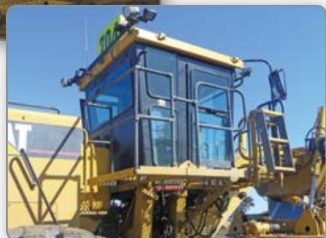
Picture 3 Access platform in the deployed position.
