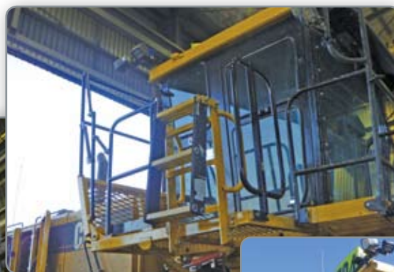
Picture 2 Rear access platform and emergency egress steps in raised position.
