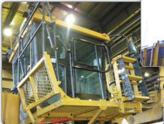
Picture 1 Rear access platform in the 'raised' position.
