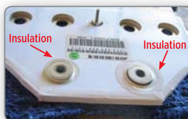
Image 2: Busbar showing insulating vinyl stickers in place.
