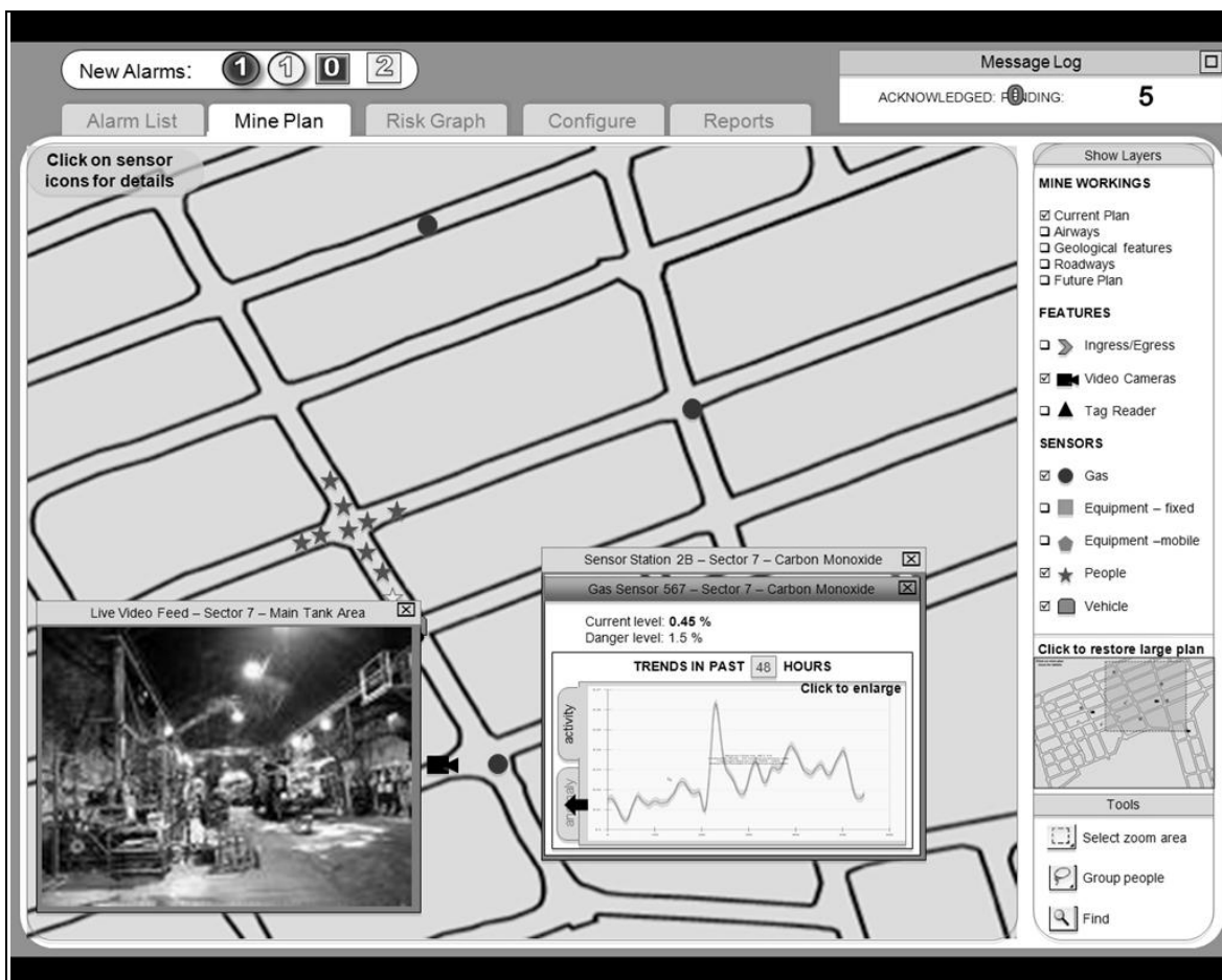
Figure 4. The Nexsys™ Mine Plan View showing live camera feeds, gas sensor locations, charted gas trends, and personnel locations.
