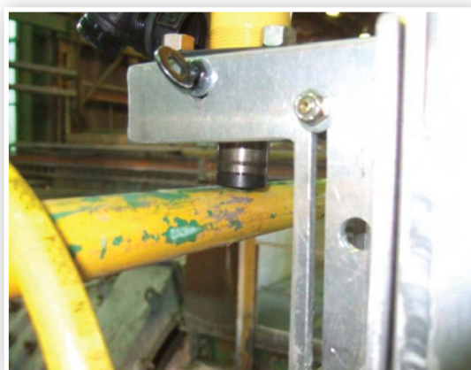
Photo 5 - Handrail tester pushing on handrail to apply correct force in the vertical plane
