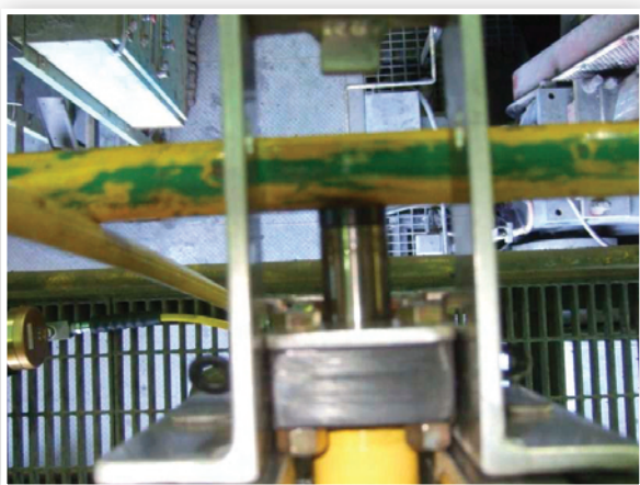
Photo 4 - Handrail tester pushing on handrail to apply correct force in the horizontal plane
