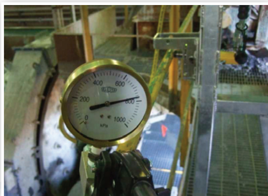
Photo 6 - Gauge to indicate that handrail tester is applying correct force
