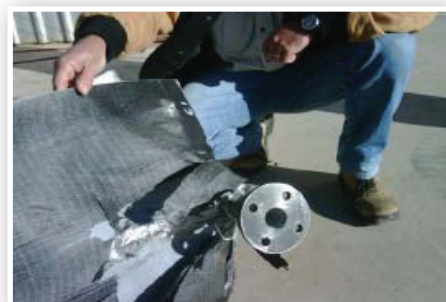
Figure 3: Post testing photos of the Kevlar panel still intact and the bent Split Set
