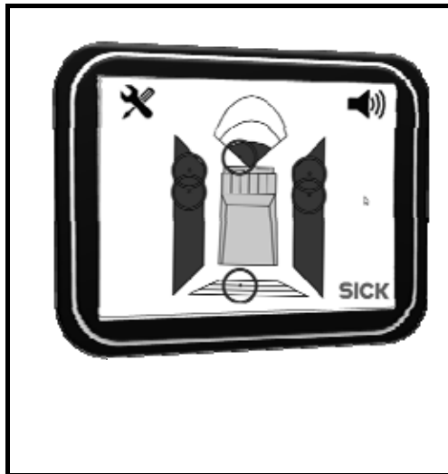
Figure 5 Operator display: warning zones with obstructions
