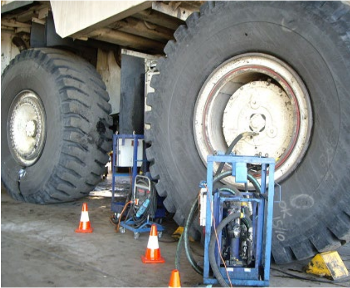
Final drives oil filtration
