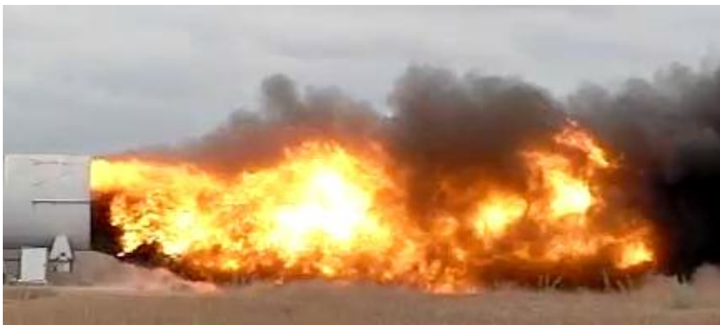
Figure 2-3 Results of a 'Seminar' coal dust explosion at Kloppersbos
