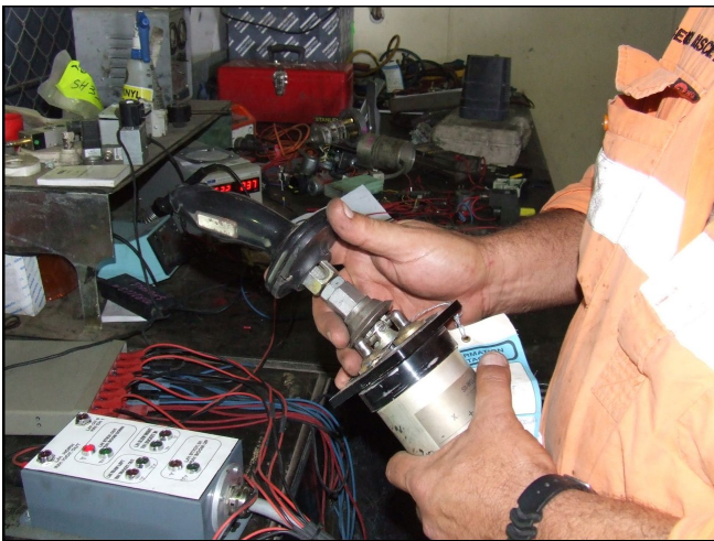
Photo 2: Once the electrician has repaired the joystick, it is connected to the system via deutsche plugs. The joystick is then manoeuvred in each direction, with LED lights illuminating in the appropriate direction if the joystick is functioning correctly.
