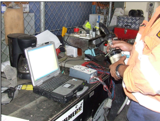
Photo 3: The electrician then connects the Joystick Test Module to a laptop to measure the voltage the joystick is operating at. This allows the electrician to use existing datalogging software to confirm that the joystick is running within appropriate voltage parameters and safe for use.
