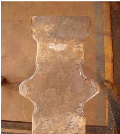
Latch lever wear before doors were realigned
