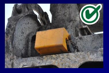
Solution - Retainment Polyurethane buffers developed for better impact qualities. Retaining lugs were cut and modified. A chain and hammer locks are now used to retain the buffer in place. These buffers last approximately **20 weeks**.
