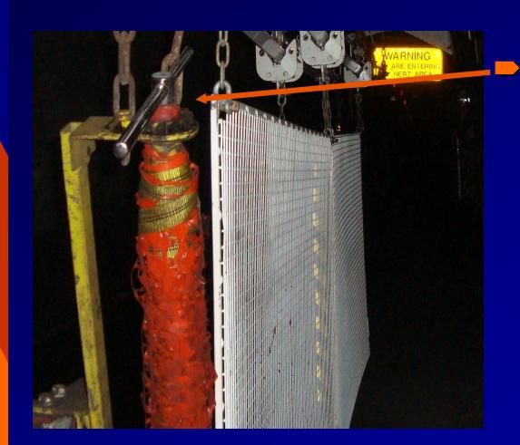
THE INBYE END OF THE MESH IS AT THE BOOT END AND IS WOUND ONTO A SPINDLE EACH TIME THE BOOT MOVES
