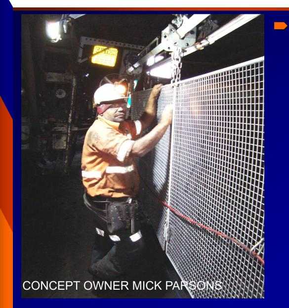
**ONCE THESE BAYS HAVE BEEN REMOVED THE BARRIER IS FULLY OPENED UP AND** LOCKED IN PLACE, PROVIDING **GUARDING TO THE EXPOSED CONVEYOR**
