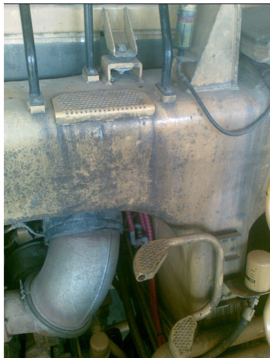
Dangerous OEM rear chassis foot peg Access
