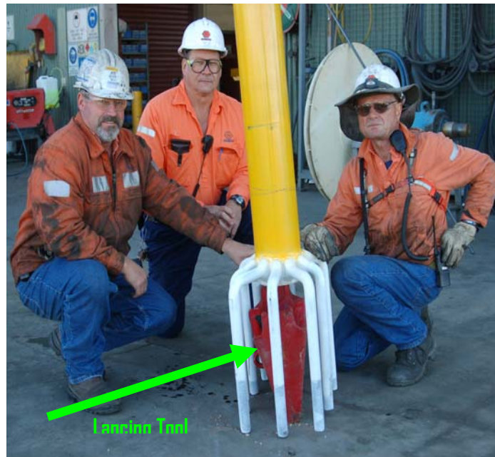
Figure 4- Use of GET Removal Tool
