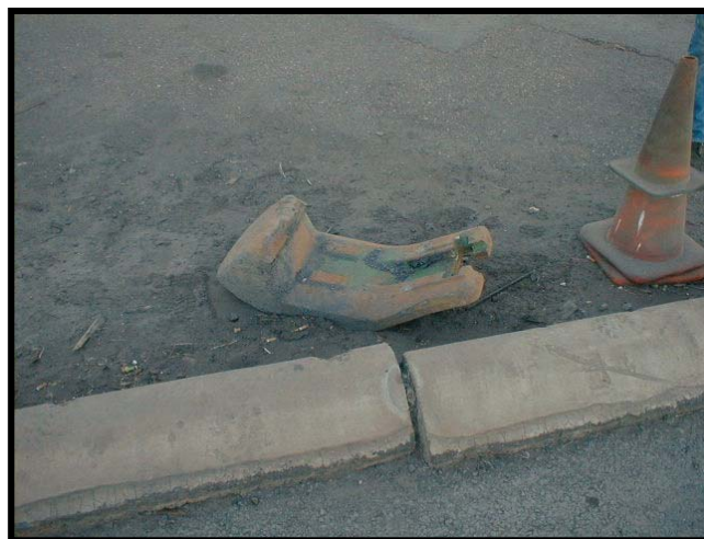
Figure 2- Typical Piece of GET Removed From Crusher
