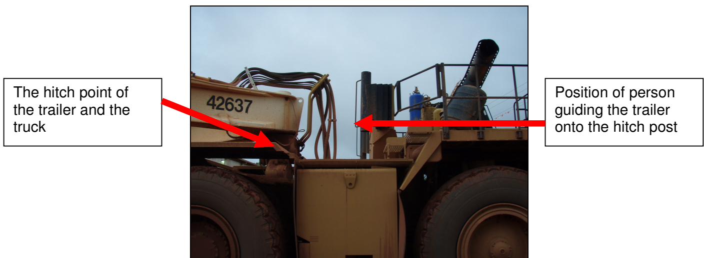
Figure 2: Side view of a haul truck and trailer at the hitch point.
