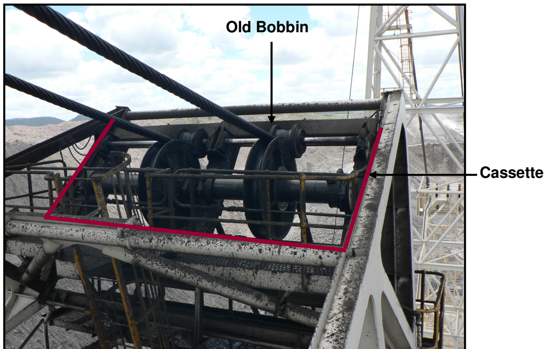
Previous cassette and bobbin roller arrangement above and below
