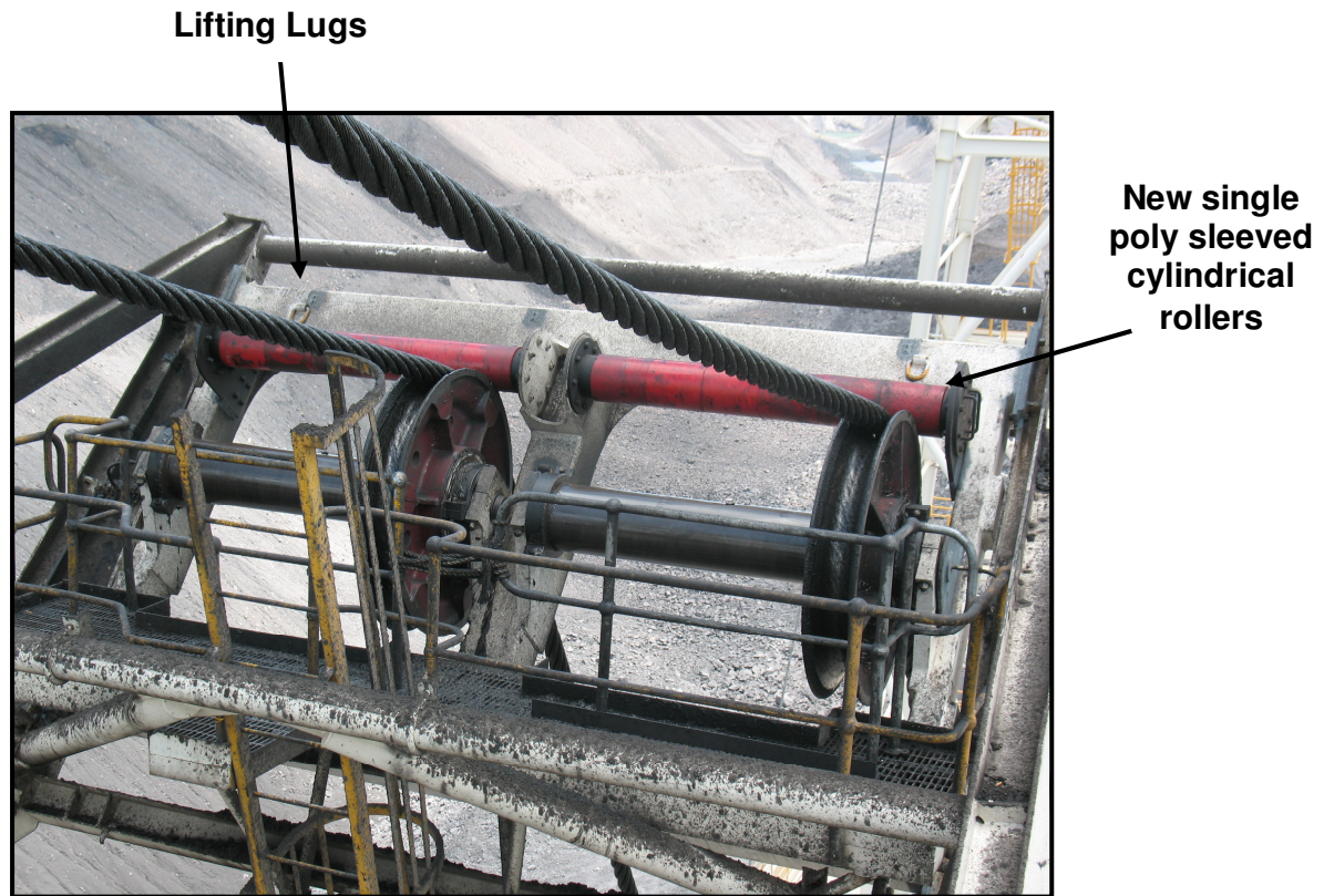
New cassette and poly sleeved roller arrangement above and below
