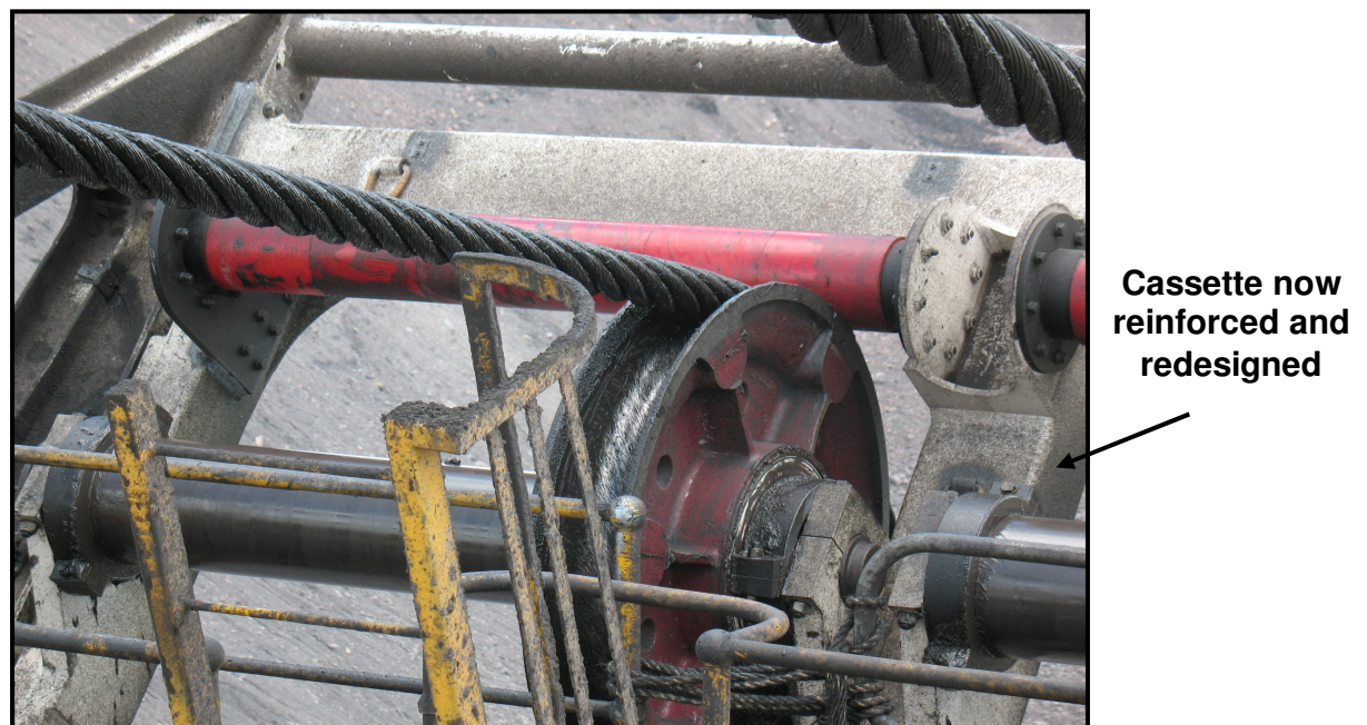
New cassette and poly sleeved roller arrangement above and below
