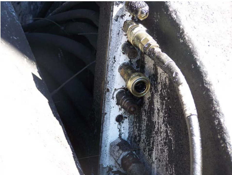
The Eimco quick coupler port The Humphrey-Guard can be attached to its relevant coupling on the Eimco ensuring correct operation.
