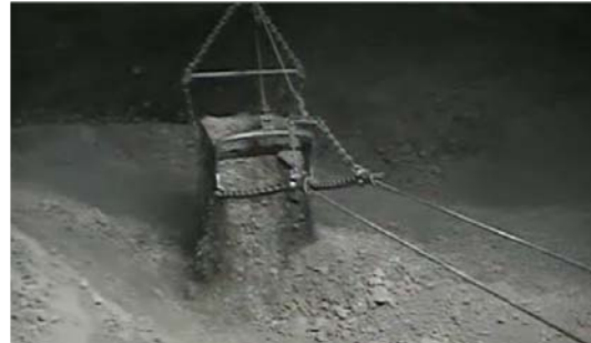
Dragline bucket location is always recorded while the machine is in operation
