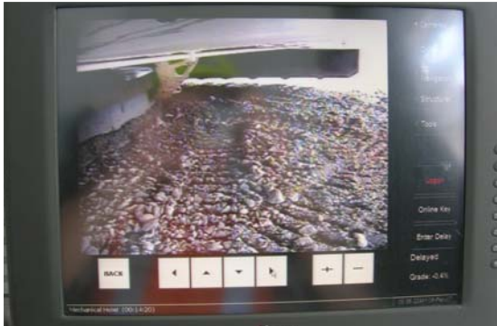
Camera display monitor in dragline cab
