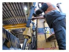
A seven month trial was held onsite to ensure that the new light bracket construction can withstand operating conditions prior to full site release. The trial has now been completed and the new lights are in the process of being fitted to the entire tracked dozer fleet.
