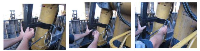
The light bracket is then lowered using the rope until it comes to rest on the step handrail allowing for maintenance work to be undertaken.
