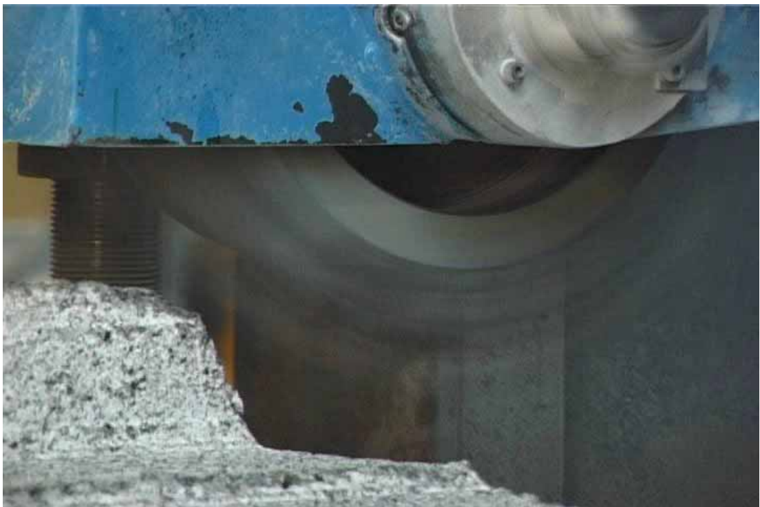
Figure 5 Cutting Harcourt Granite
