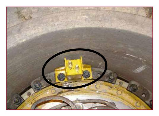
VPS installed on 830E, secured to existing wheel studs
