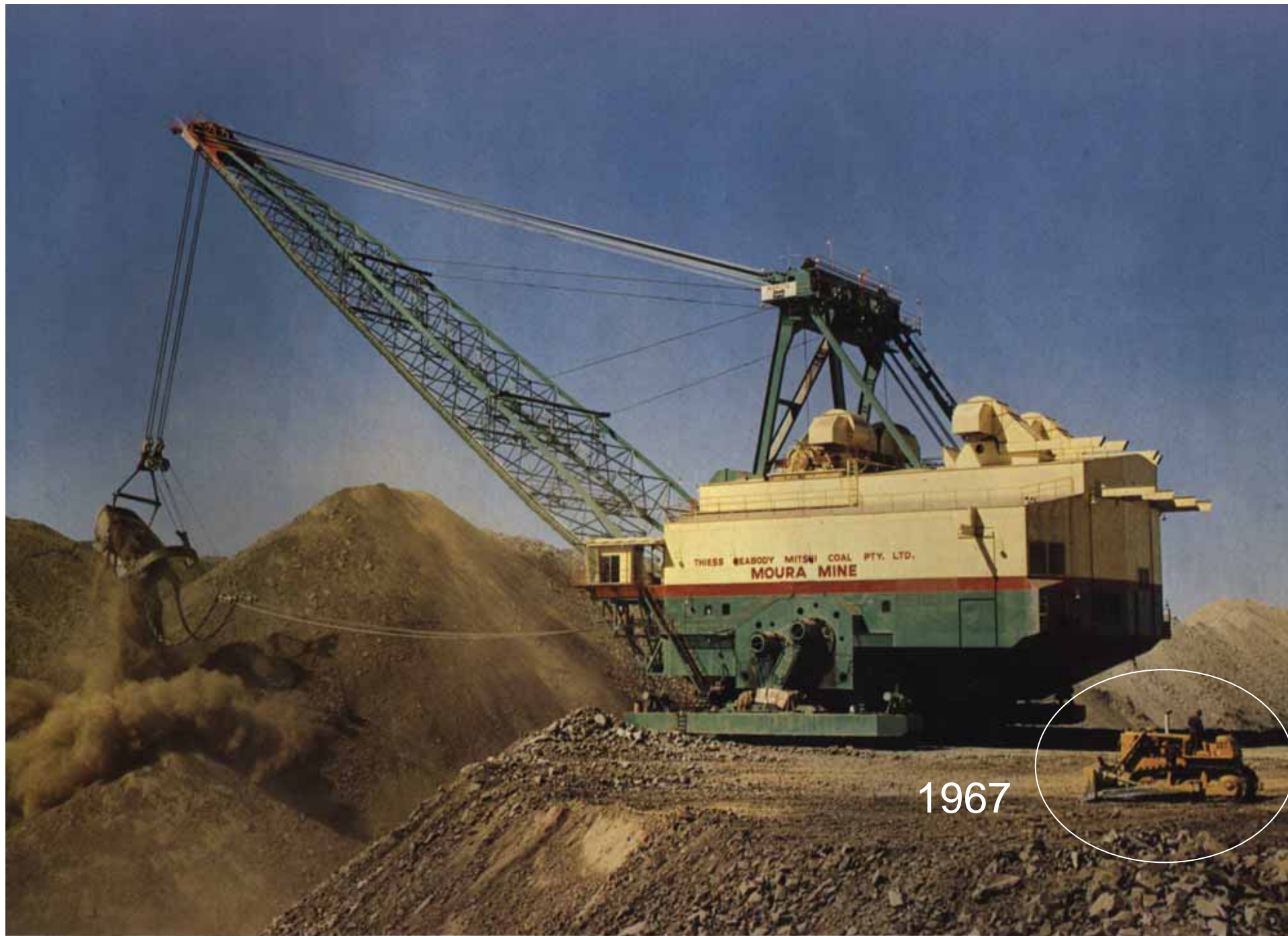
Marion Type 8900 Dragline—130 c.y. Bucket, 275' Boom, 18,000 A.C. h.p., 13,239,000 lbs. Working Weight
