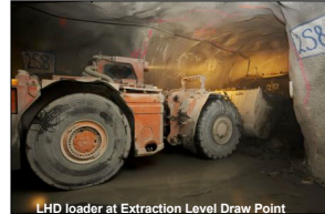
LHD loader at Extraction Level Draw Point
