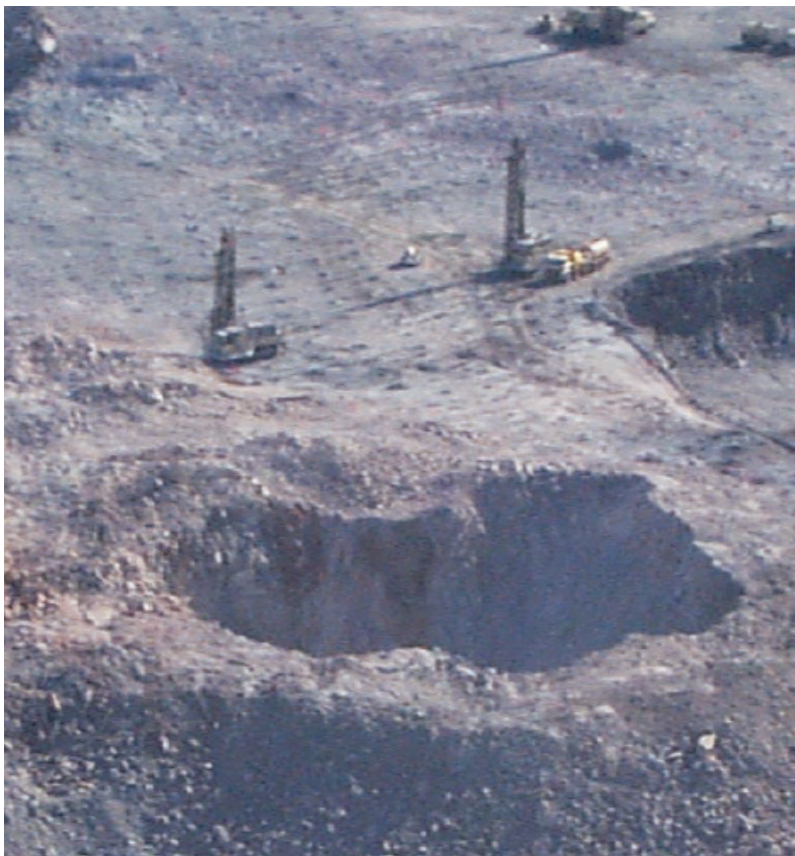
Figure 3 Voids from old workings at a West Australian Gold Mine.
