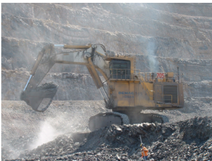
Figure 1 GPS systems such as this APS installation on an excavator at Century Mine can largely eliminate the need for people on the ground.
