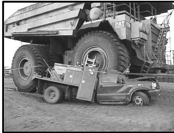
Figure 9 Damage inflicted on a light vehicle when run over by a haul truck
