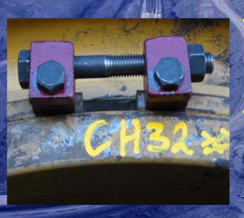
Lock Rings are held together with a strong easy to install retainer
